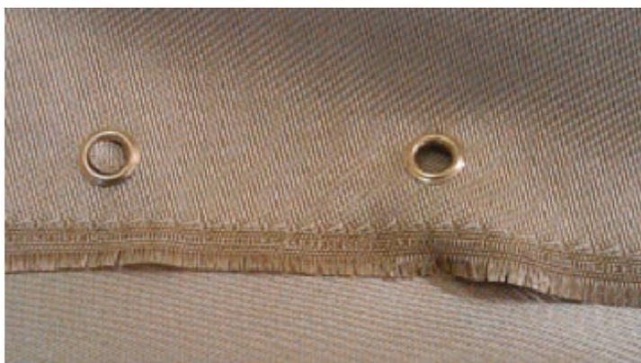
Silica fabrics can be used for welding blankets, fire blankets, fire curtains, stress relieving blankets, flexible connectors, furnace curtains, gasket materials in valves controlling the flow of molten alloys, etc.
