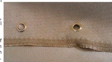
Silica fabrics can be used for welding blankets, fire blankets, fire curtains, stress relieving blankets, flexible connectors, furnace curtains, gasket materials in valves controlling the flow of molten alloys, etc.
